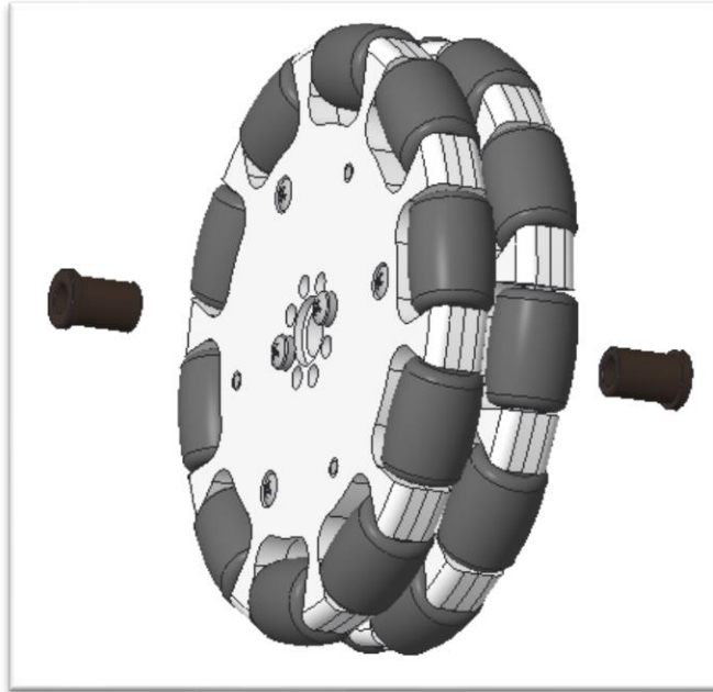
Figure 35- Unassembled view of singular wheel assembly, perform this step on both assemblies
