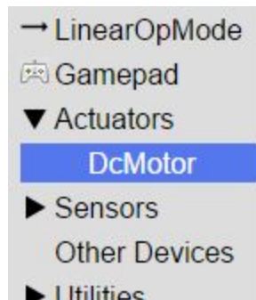
Figure 70 - Only the DcMotor subcategory is available for our Op Mode since we only have a motor controller configured.
