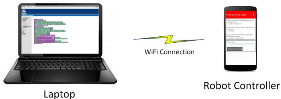
Figure 35 - The laptop communicates with the programming server through a wireless connection.
