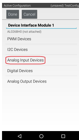
Figure 135 – Touch “Analog Input Devices” to configure the analog sensor that is connected to this module.
