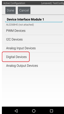
Figure 137 - Click on Digital Devices to edit the digital sensor information.
