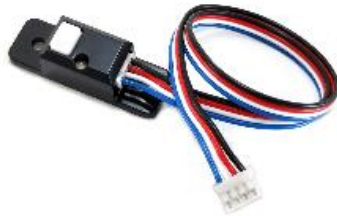
Figure 9 - REV Robotics Touch Sensor.
