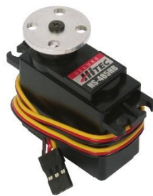
Figure 6 – An example of a servo motor that is commonly used on FIRST Tech Challenge robots. 6
