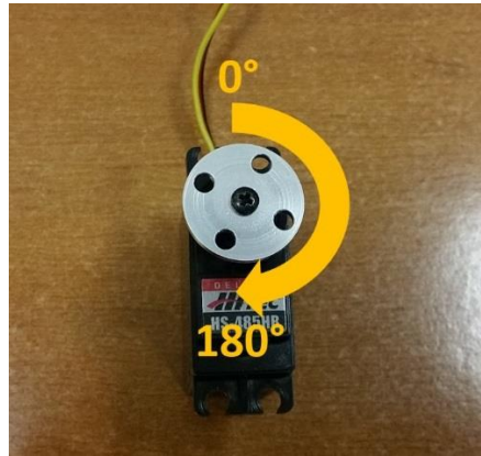
Figure 7 - A typical servo motor can rotate to and hold a position from 0 to 180 degrees.
